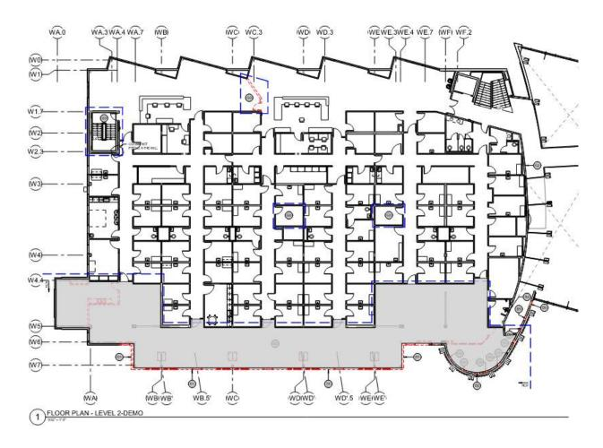
GRAPHIC TO SHOW EXTENT OF CEILING DEMO LEVEL 2 - PER BIDDING QUESTION: "Can the Architect provide a Reflected Ceiling Demo Plan that shows the extent of ceiling demo?"
