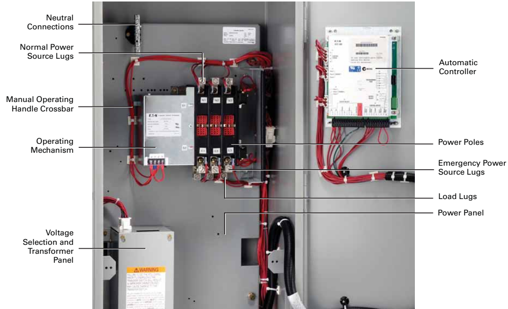
Typical Contactor-Based ATS 100–400 A
