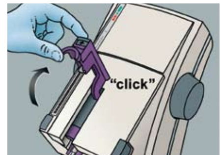
Fig. 9 Locking lever snaps into the uppermost position.
