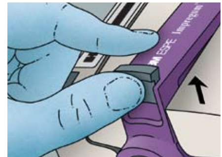
Fig. 8 The locking lever can be opened (to change mixing tip) while the cover of the Pentamix™ 3 Automatic Mixing Unit is closed.
