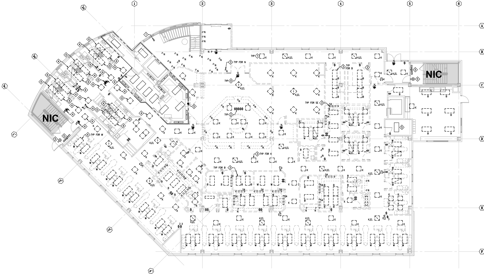
1 DEMOLITION FIRST FLOOR PLAN - LIGHTING ED102 SCALE: 1/8" = 1'-0"
